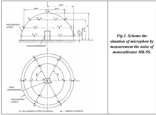
These engineering methods are designed for certification of production attitude of the emission noise. They are used for a measurement of the level of the noise in exploitation circumstances.
