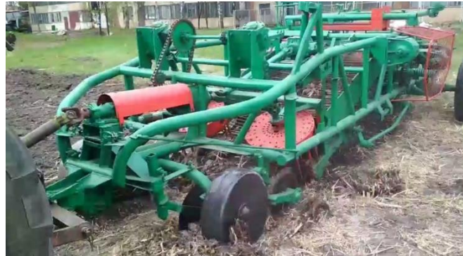
Fig. 6. Machine for digging up miscanthus rhizomes during the field experimental investigations
