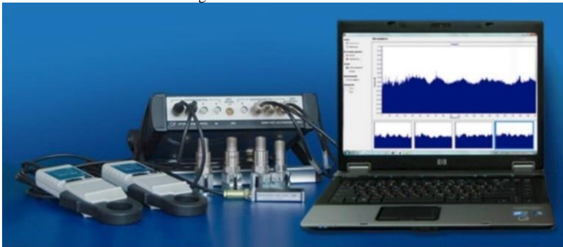
Fig. 1. An example of the implementation of the measuring system of currents and voltages of the stator circuit AM
