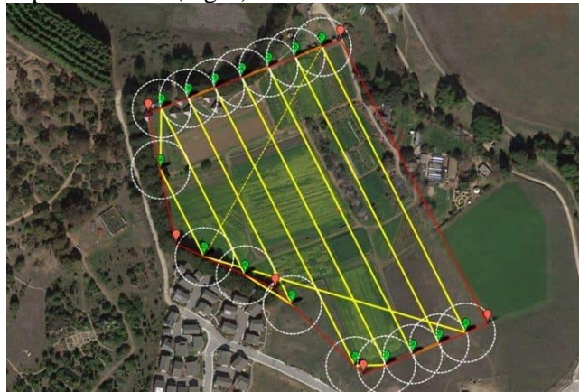
Fig. 7. An example of a UAV flight route when planning a terrain survey
