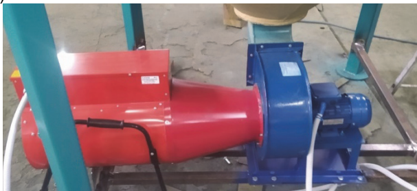
Fig. 9. General view of convective walnut dryer. a – the front view, b – the screw working body, c – system of air flow heating and injection into the drying chamber
