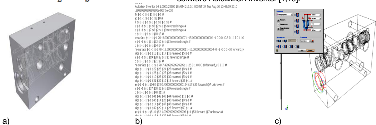
Fig. 1. Electronic image of the part a) - 3D model of the distributor housing; b) - fragment of a text file, c) - parametric model of the corpus; containing a description of the geometry and elements of the part
