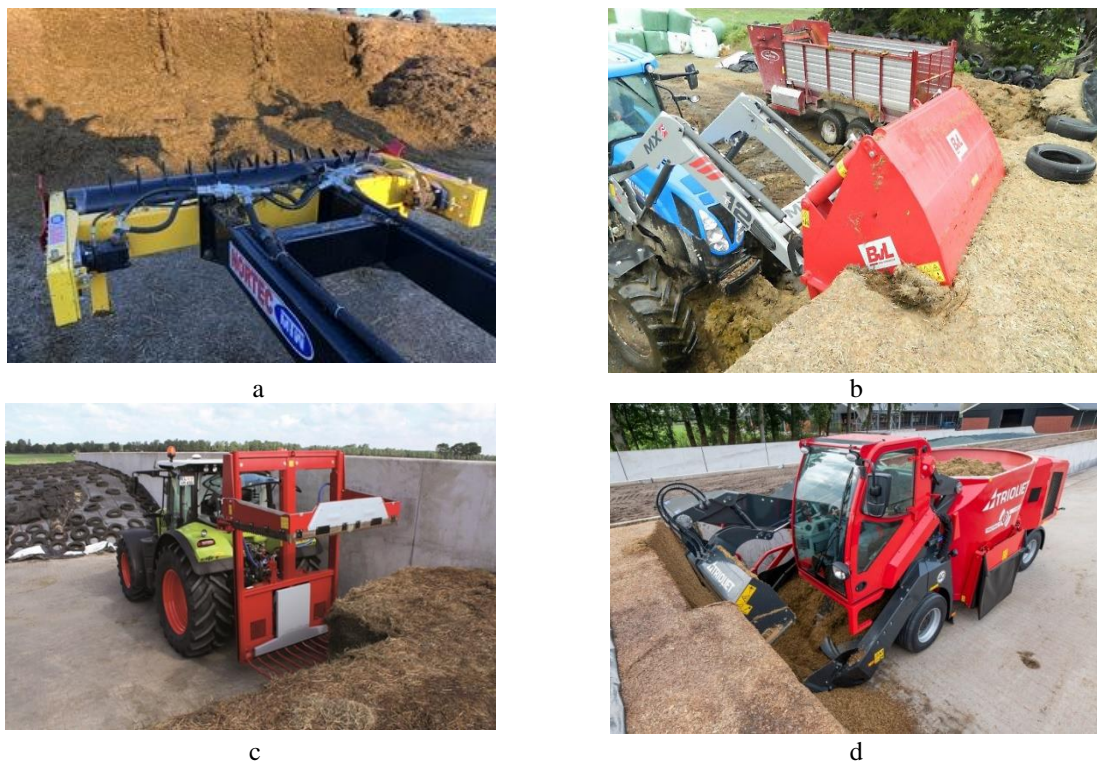
Fig. 1. Loaders of stalk feed from a silage trench: b – cutting grip V-LOAD Shear (Germany), c – forage cutter V-Load Cutter BVL (Germany), d – feed mixer Trioliet Triotrac M (Netherlands)
