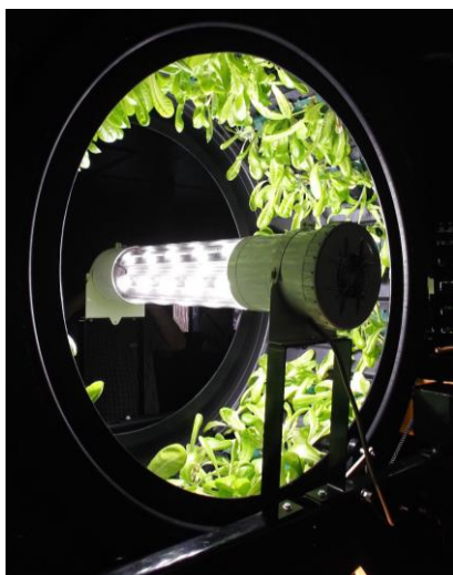
Fig. 5 The scheme of a rotary hydroponic system
