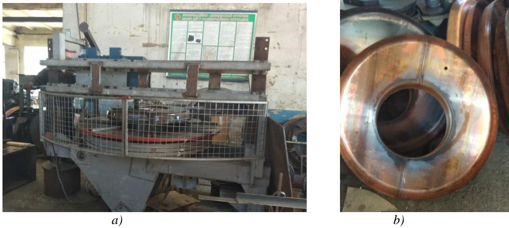
Fig. 3. Assembled representation of the SR installation: a) formation of inner flanges on the lid of the fermentation column; b) appearance of the lid of the fermentation column with the formed inner and outer flanges
