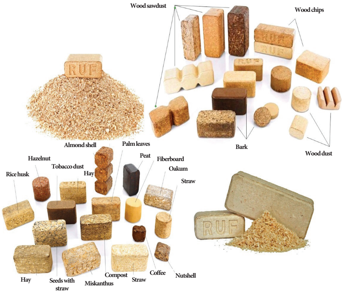
Fig. 8. General view of fuel pellets from biomass
