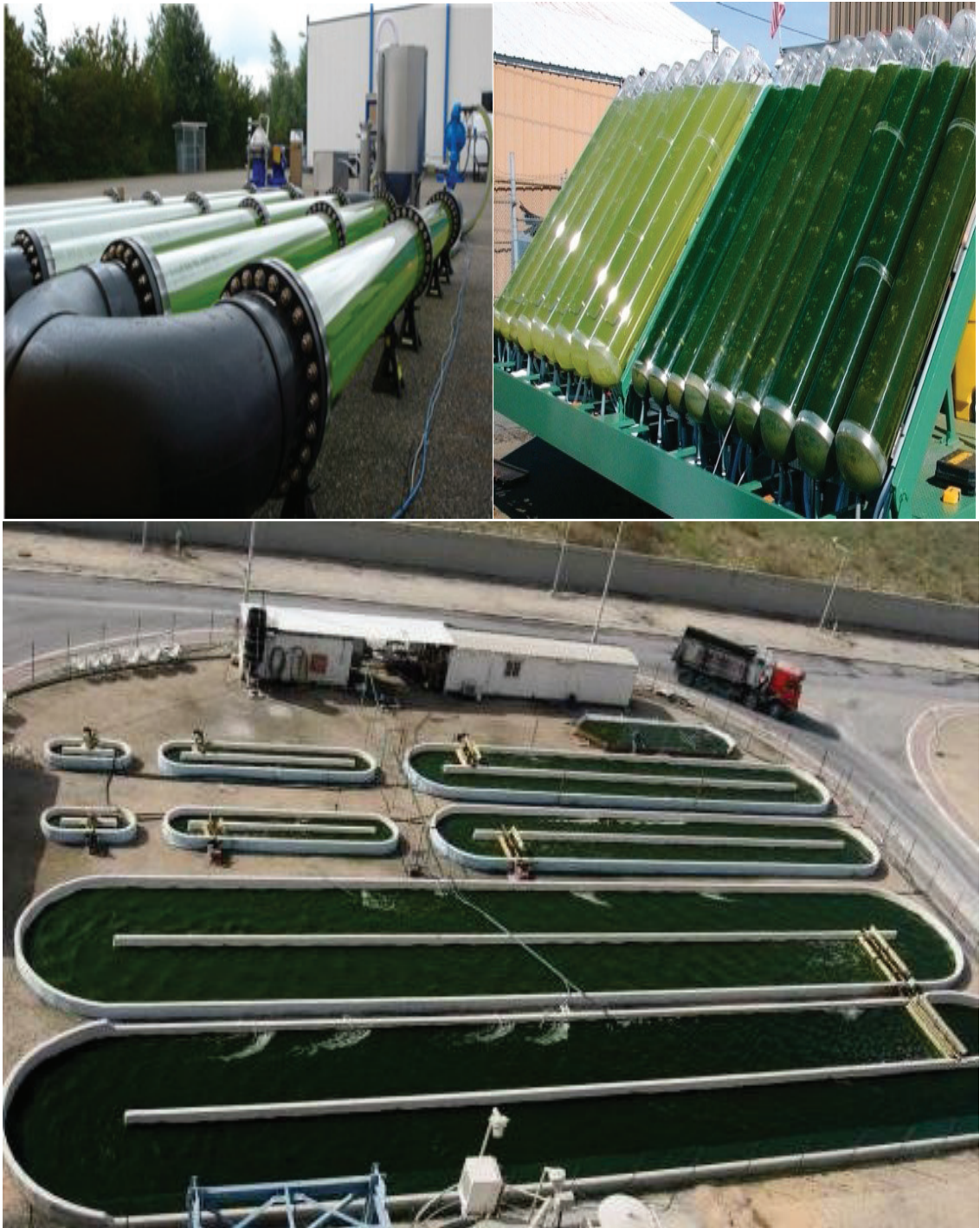
Fig. 2. Bioreactors and open water reservoirs for microalgae growing
